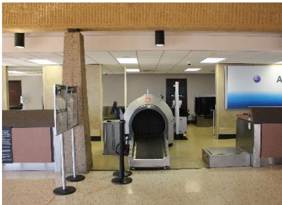
Figure 2-25. Bag screening machine CT-80
